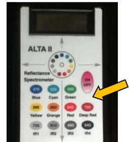
2. Hold the instrument so that your group can see inside the lamp/sensor array on the back of the instrument. **BE CAREFUL NOT TO PLACE ANYTHING INSIDE THIS OPENING.** Press and hold the blue button on the front of the instrument. You should see the blue lamp glow as long as you continue to press the blue button. When you release pressure the lamp shuts off.
